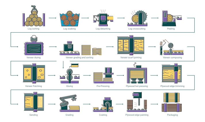
The birch logs are debarked and cut into shorter lengths. Then, they are rotated on a lathe, and a sharp blade peels 1.5mm veneers. The veneers are then dried in a kiln to reduce their moisture content, preventing warping and ensuring proper bonding in later stages.
